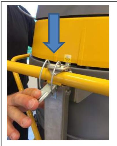
During transport the transport bracket / handle MUST be locked.
