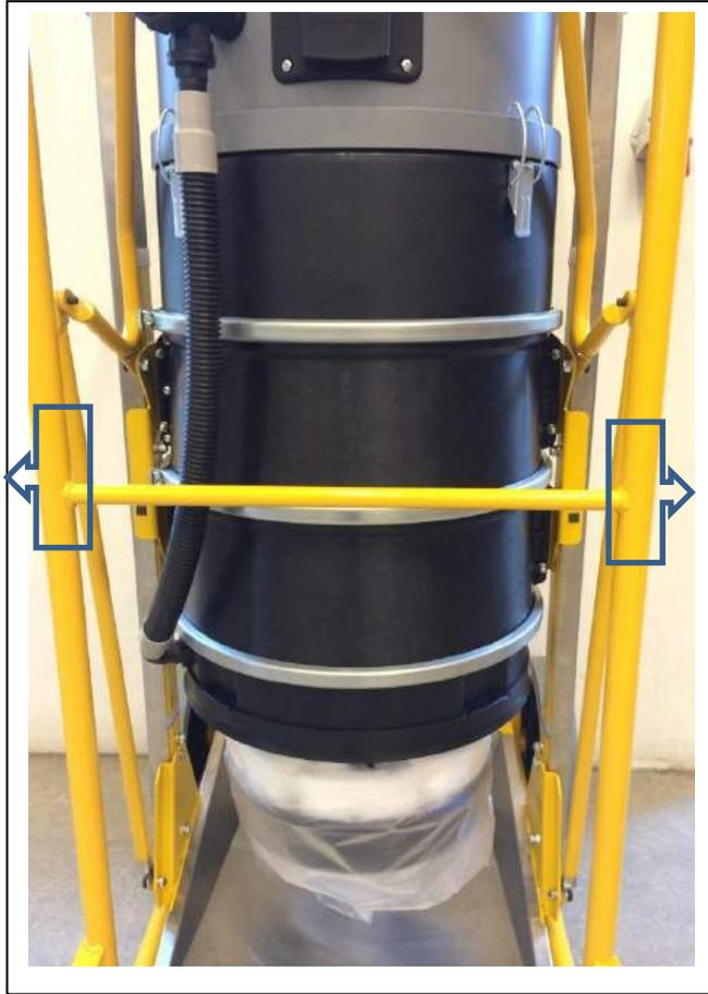
The machine is transported standing. Clamping etc. only round the cross bar at the front of the frame. SEE THE MARKING IN THE PICTURE TO THE LEFT. MAX. traction 10 kg.
