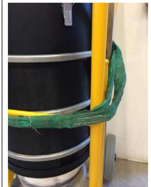
Besides make sure that the wheels and the back of the frame have a fixed installation in the car so that the frame is not tightened in a lopsided way or will tip over during transport.
