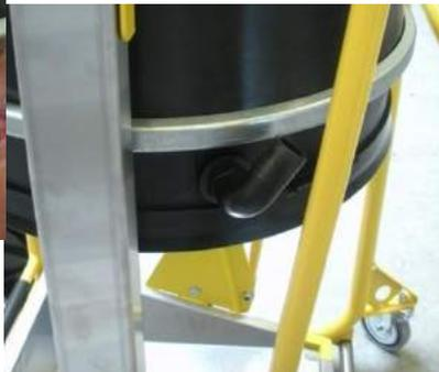
Unscrew the blind plug and mount the hose connector with the washers enclosed.
