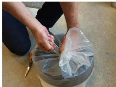
This will be the beginning of your bag and the bottom. Be aware - when collecting heavy materials - that this cable tie is to hold the total weight of the material collected. Be sure that the cable tie is tight - otherwise it can fall off.
