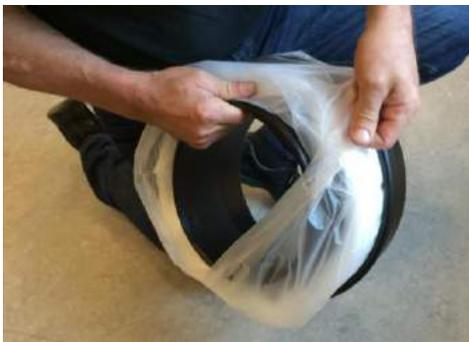
Check that the bag does not fold or in any other way prevents the Longopac from being pulled freely out
