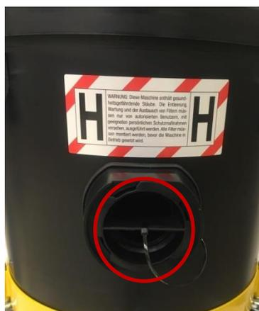
The container is equipped with a plug which is to be used during transport and whenever the machine is not operating.
