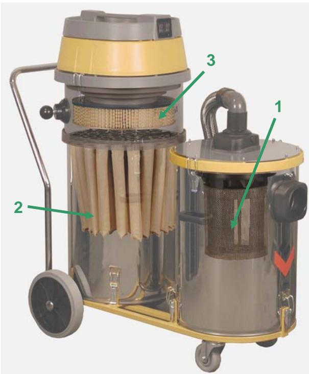
A strong wire grating (1) in the cyclone separator in container 1 holds back the large particles, and because of the cyclone effect in the container also a large part of the small particles will be held back. In container 2 the large multi-tube filter (2) is made of a fire-resistant filter material.
