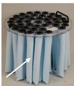
The large multi-tube filter in RONDA® 2-58 Duo is mounted in container 2. The multi-tube filter has been tested with quartz-dust-particles of which more than half is less than 5  $\mu\text{m}$ . (5  $\mu\text{m}$  correspond 0.005 mm.) The filter holds back 99.97% of all the particles, which corresponds to an emission of 0.06 mg/m<sup>3</sup> in the purified air.
