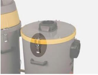
Release the lid of container 1 by loosening the two container clips that secure the lid.
