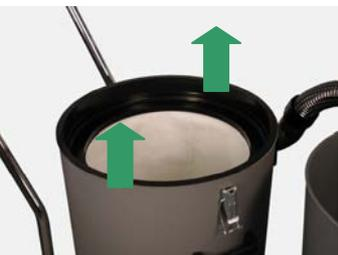
Lift the standard filter/multi-tube filter out of container 2. Remove the filter from the container by lifting in the black mounting ring. Use the two black lifting handles at the top of the filter plate to remove the multi-tube filter.
