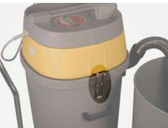
Empty container 2 by first removing the motor top. Loosen the two container clips securing the motor top on top of container 2.
