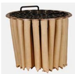
The filter consists of a large number of tubes mounted on springs. During operation the tubes move, and some of the dust that can stick to the surface of the filter will fall down into the collection container.
