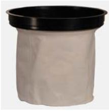
The standard filter is held in place by the deflector under the motor top. The filter holds back the fine and smallest dust particles and protects at the same time the turbine blades of the two suction motors. The turbine blades may be damaged if there are wearing particles in the air current.
