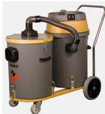
RONDA<sup>®</sup> 5-58 Duo has 2 separator containers. Container 1 is a cyclone separator with a coarse filter and separates liquids, coarse particles, chips etc. larger than 1.5 mm. Only the finest dry particles will continue to separator container 2.
