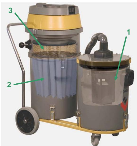
1: The pre-filter is placed in container 1 and is secured on a black mounting ring placed immediately under the lid of the container. The float valve, which is mounted at the lid of the container, keeps the filter stretched.
