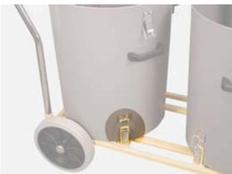
Release container 2 by loosening the three clips that secure the container to the trolley frame.
