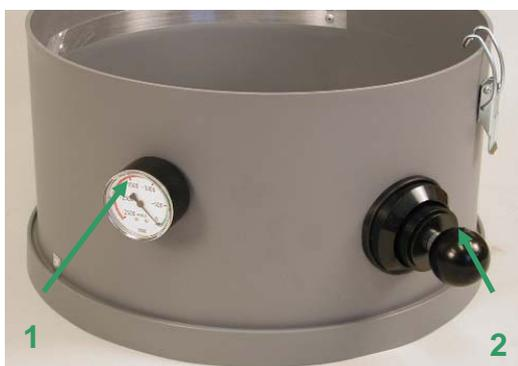
The manometer (1), which is placed on the adaptor ring, measures the atmospheric pressure in the machine during operation.
